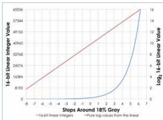
Fig 1: The raw data from a video sensor is linear, but calculating a log of that value gives a much more even spread of picture information from stop to stop.
