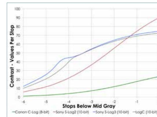
Fig 5: Contrast in the shadows – a higher line means more detail stored, but noise will be more obvious before correction. The Canon line is low because the C300 records 8-bit; the 10-bit curves exceed Canon's stop zero (18% gray) value deep in the shadows.
