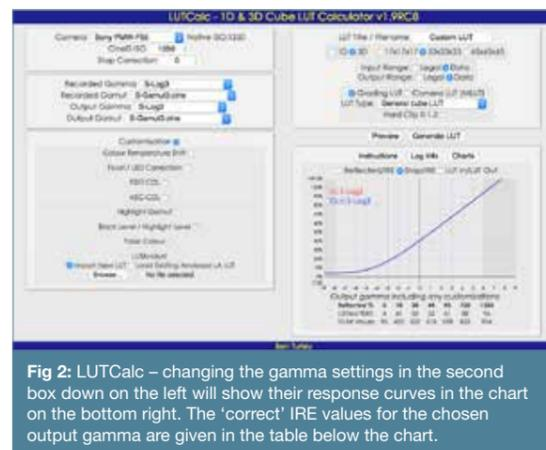
Fig 2: LUTCalc – changing the gamma settings in the second box down on the left will show their response curves in the chart on the bottom right. The 'correct' IRE values for the chosen output gamma are given in the table below the chart.
